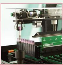
The samples selected for ESR testing are transferred from the "Preparer Module" to the "Analysis Module" where the test is executed in four steps: mixing, first reading, sedimentation (20 minutes), second reading. To ensure traceability, each sample is placed in a specific position of the Sample Holder Rack.
