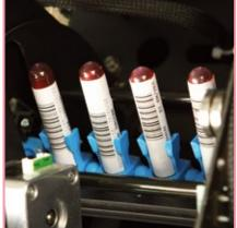
ESR results for each test are obtained using standard ESR test methods (three phases: rouleaux formation, sedimentation and packing). These results, obtained in 20 minutes, correlate with the Westergren citrate reference method (a 60 minute test performed at 18° C). Results from the Ves-Matic Cube 200 follow ICSH recommendations (J Clin Pathol 1993; **46:** 198-203)
