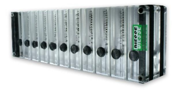
Manual system for the determination of the ESR on 20 samples simultaneously, using all models of DIESSE tubes (VacuTec - VacuCode - VesTec)
