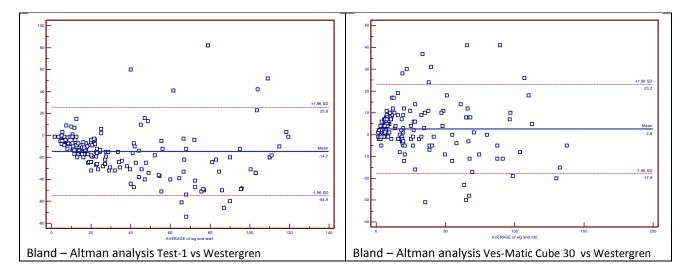
Test-1 vs Westergren: limits of agreement -54,9 ÷ 25,6 mm/h, bias = -14,7 mm/h Ves-Matic Cube 30 vs Westergren: : limits of agreement -17,9 ÷ 23,2 mm/h, bias = 2,6 mm/h The limits of agreement for the Test-1 are roughly the double of those for the Ves-Matic Cube 30. The **Spearman's correlation coefficient** was 0,85 (CI 95% 0,80 ÷ 0,88, p<0,0001) for the Test-1 and 0,91 (CI 95% 0,85 ÷ 0,94, p <0,0001) for the Ves-Matic Cube 30.
