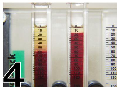
8. Repeat the reading, making sure to not excessively move the Ves-Rack II containing the samples during the reading.
