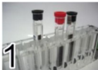
2. Place the bottom of the rack on the palm of the hand, grip it well. Turn it upside down slowly at least 20 times, in order to obtain a perfect homogenization of the samples, making sure that the air bubble moves through the cuvette at every inversion (Fig. 2).
